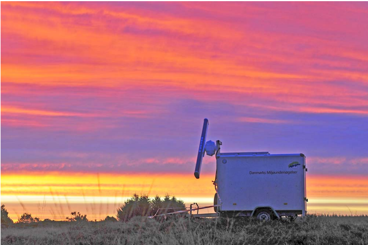
Figure 3. Vertical radar is used to provide data on flight altitude of nocturnal bird migration in the study area. © Henrik Haaning Nielsen.
